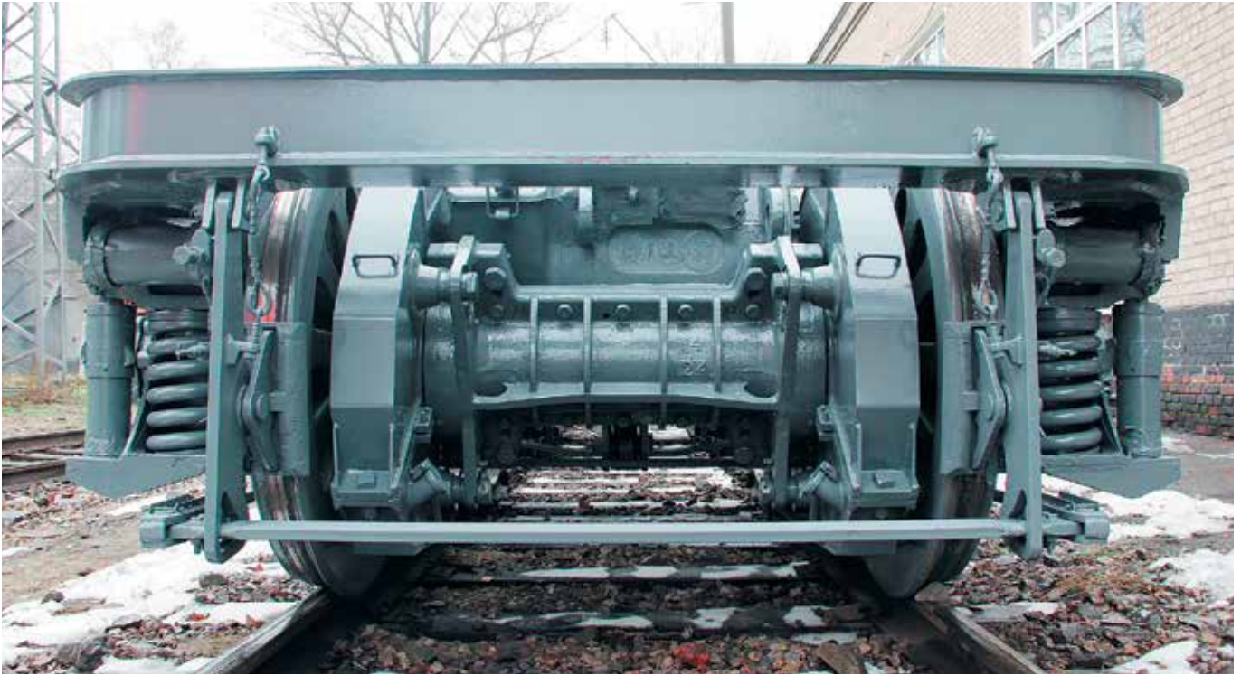
Bogie with rolling axle wheels and motor unit
