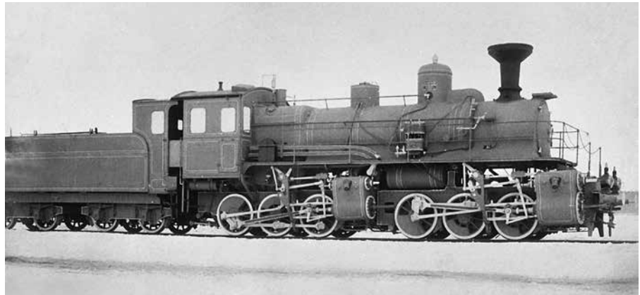
Duplex steam locomotive with six axles and frontal swivel bogie
