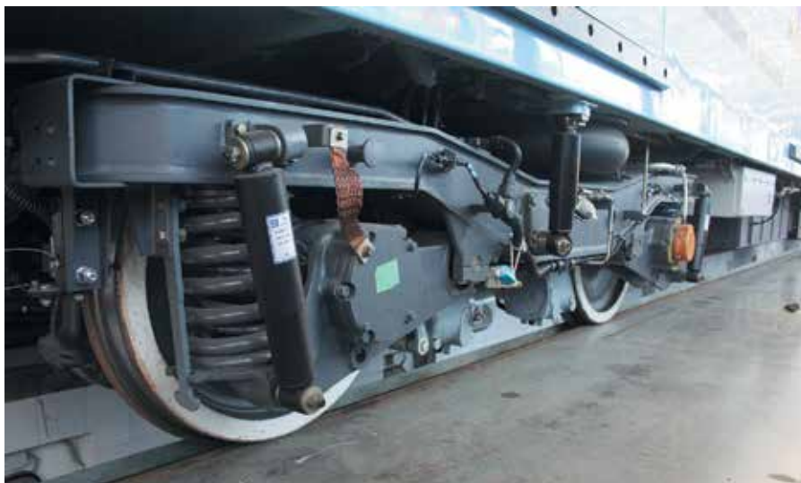
Bogies with air-ride allow for soft and quiet train movement
