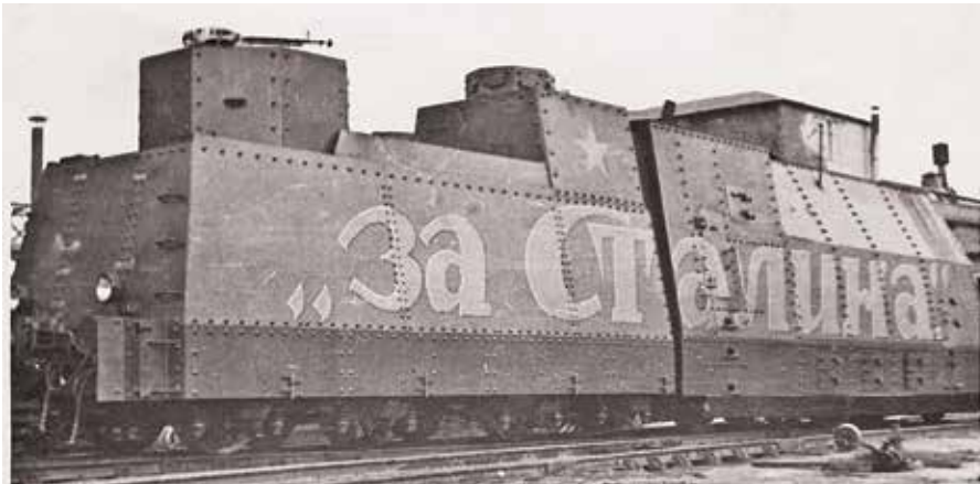
9P locomotive with a tender after armoring
