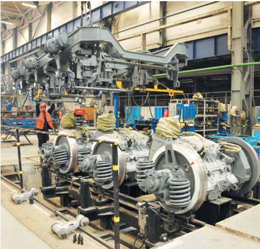
Bogie manufacture is coming to an end. Workers are getting ready to lower the frame onto wheel and engine units
