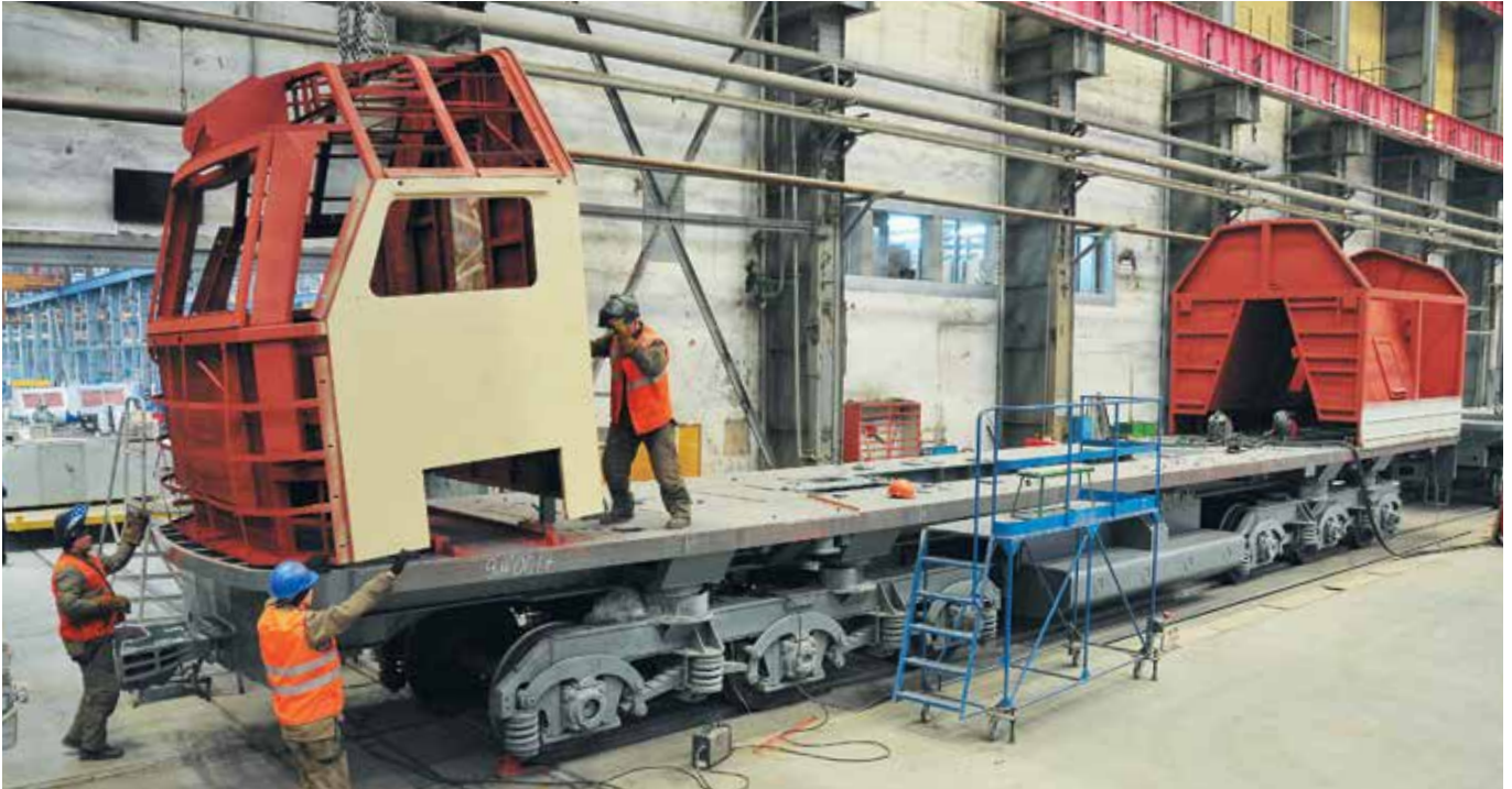
The driver's cab as one of the main assemblies of a locomotive is among the first ones to be installed onto the frame
