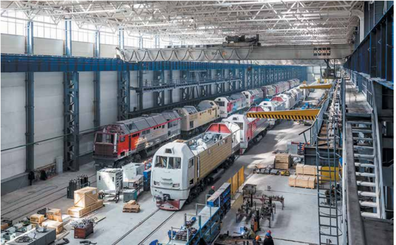
Diesel locomotive assembly, testing and fit-out line
