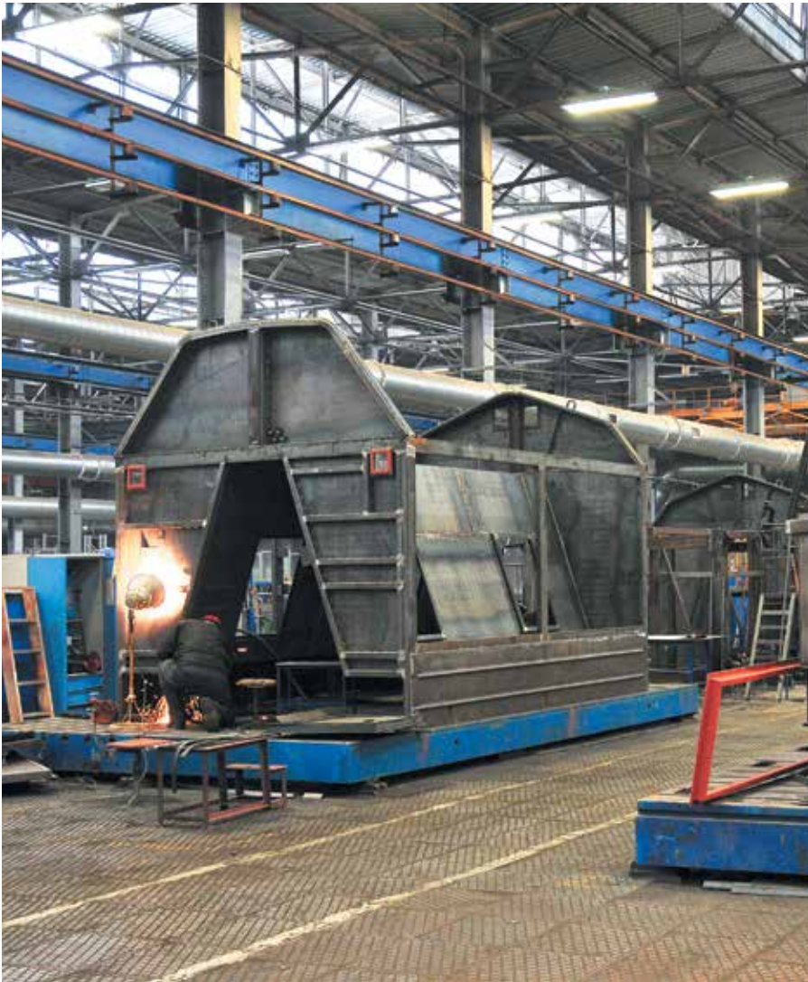
Refrigerator being designed. It will take its place on the diesel locomotive's frame
