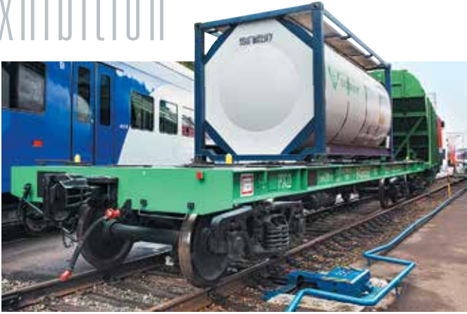
Transmash plant from the Saratov Region brought to the exhibition a new platform that may be used for transportation of both tanks and containers
