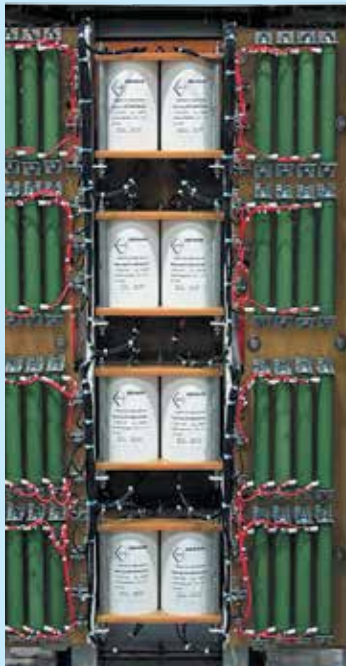
Power unit (PU) consisting of two absolutely identical channels (No. 1 and No. 2)
