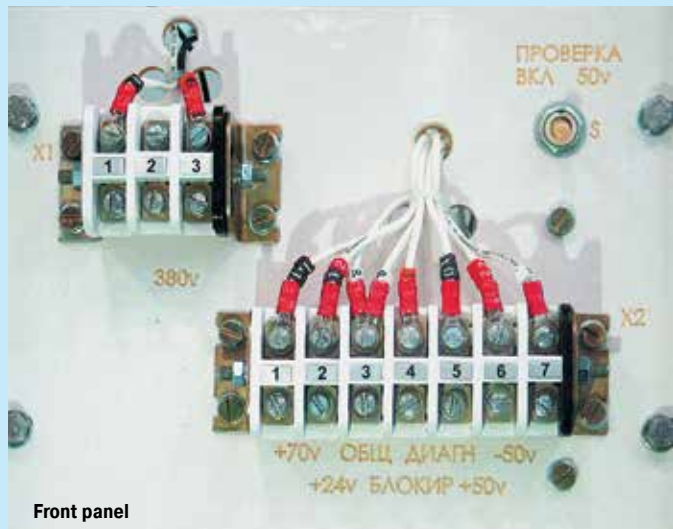
Power supply unit (PSU) which supplies power to controls units (CUs) and diagnostic units (DUs)
