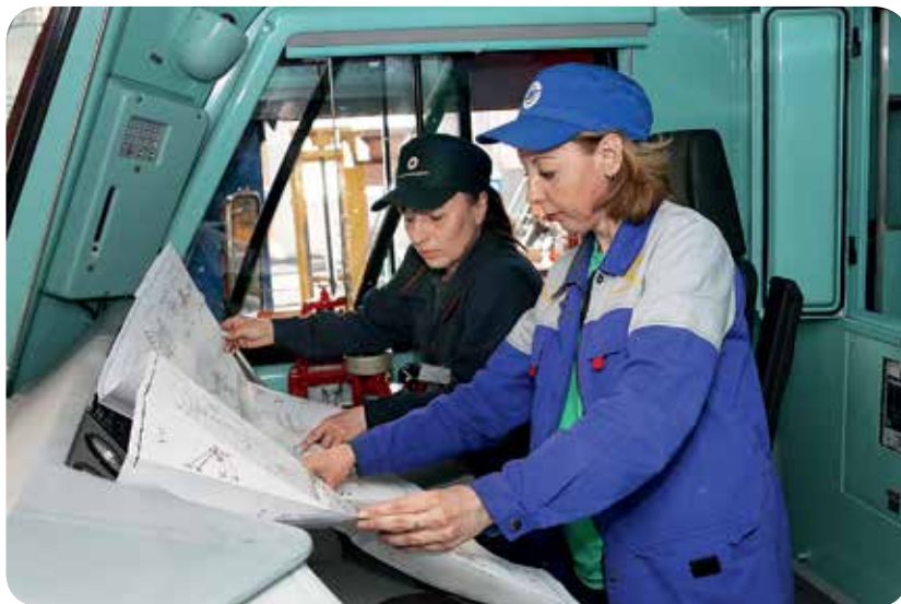
Control of installation of units in the cab of the 3ES5K electric locomotive
