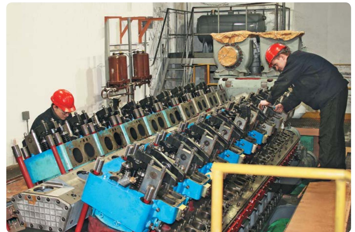
Assembly of the 20EDG500 diesel generator for nuclear power plants
