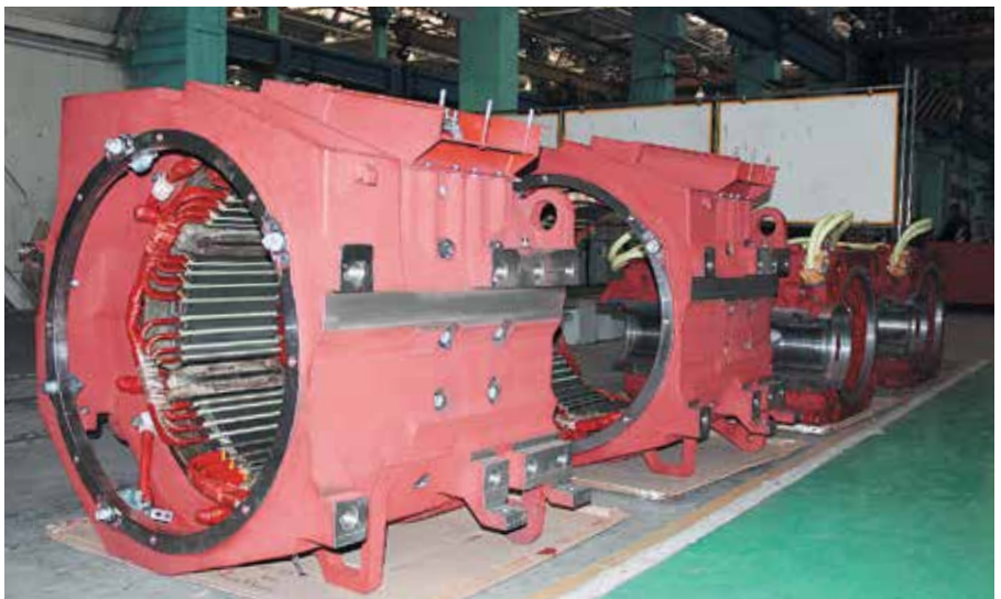
Motor frames together with pole systems, in the foreground — DTK-800, in the background — DTK-417TS
