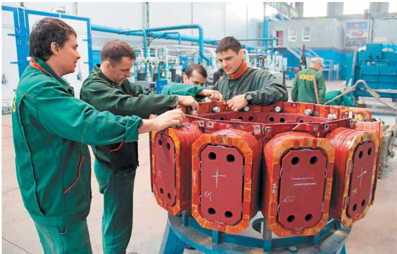
Assembling a generator rotor core
