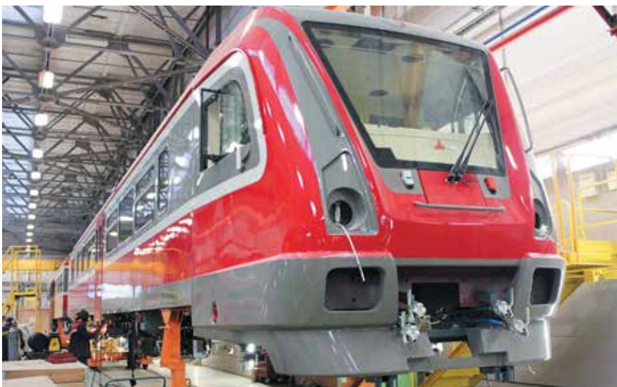
Assembling of the diesel train in the Metrovagonmash shop
