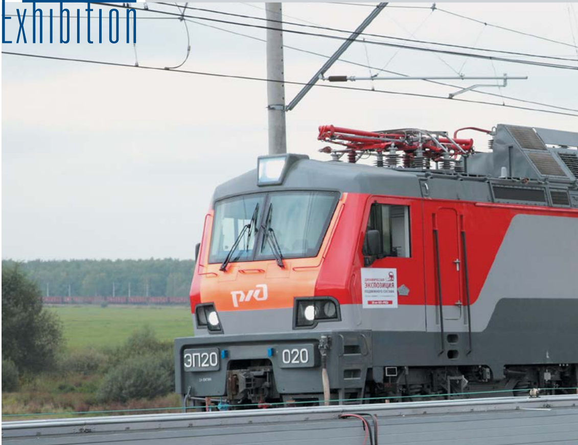
Over two dozen EP20 dual-system electric passenger locomotives have rolled off assembly lines
