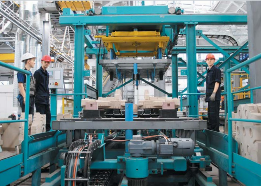
Casting molds produced on the automatic molding line
