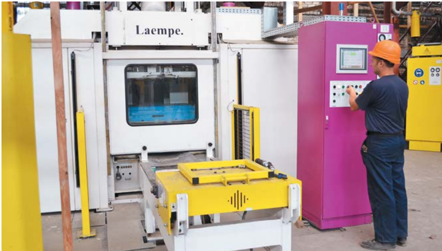
Production of rods using a Laempe rod machine
