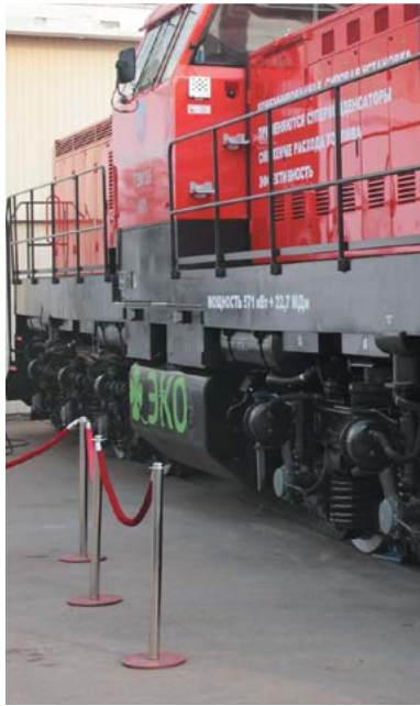
▶ TEM33 and TEM35 locomotives are highly unified with interchangeable modules
